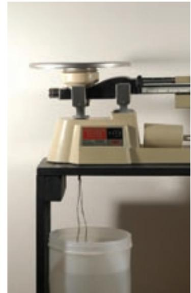
Weighing paperweight in air (left) and while submerged in distilled water (right)
